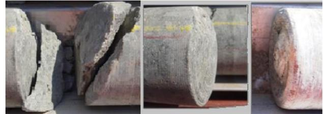
Figure 9: Core grinding from incipient through to a full grind. (Photo courtesy Debswana)
