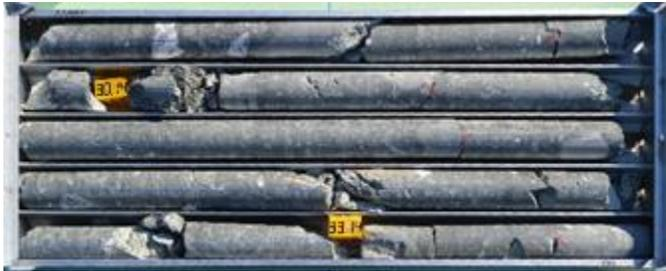
Figure 1: A core tray with depths written on core blocks separating the core recovered from each drill run.
