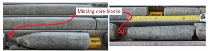
Figure 5: Tapered core segments indicating runs were made-up to achieve a near constant advance. (Photo courtesy Debswana)
